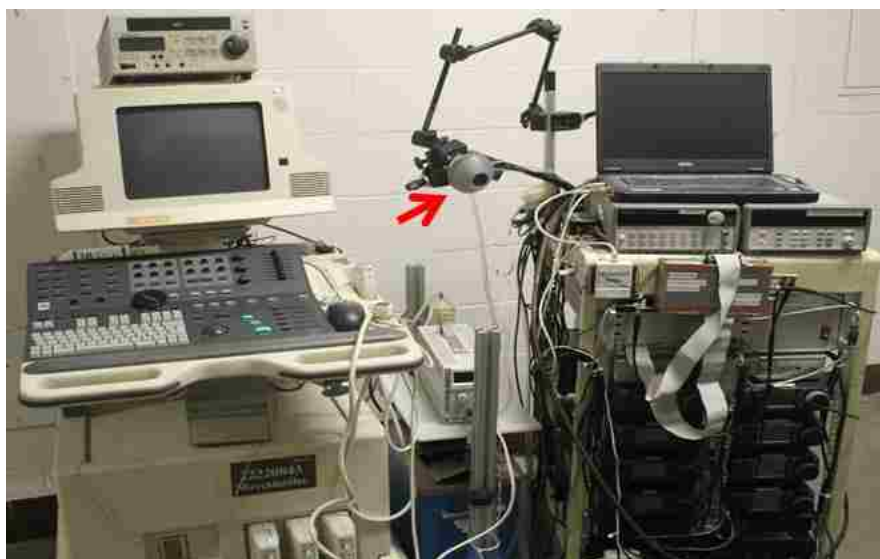
FIGURE 5.1: Image showing the first generation array device used in the threshold study. On the left is the HDI 5000, which collects an image of the kidney with a coaxially aligned P4-2 transducer. In the middle is the water cooling and circulation system, and on the right is the custom-built array device. The red arrow indicates the 2 MHz array transducer with the water-coupling cone.
