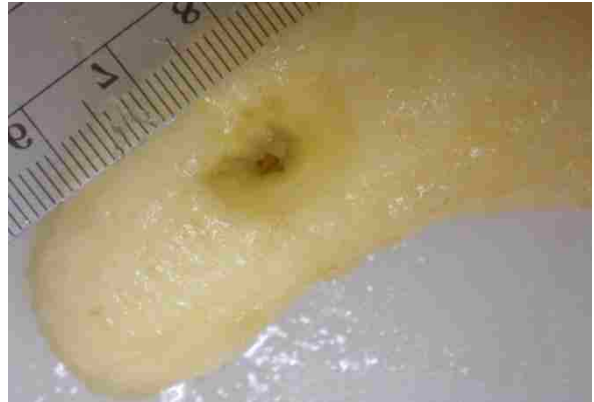
FIGURE 3.5: Photograph showing surface erosion after atomization of a banana. The hole in the banana is quite large compared to the tissues even though the exposure parameters were similar (10-ms pulses at a 1 Hz pulse repetition frequency).
